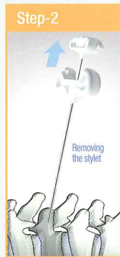
Pull the stylet out the bone puncture needle(SWMVP)
